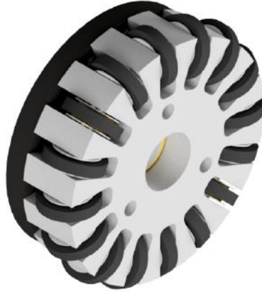
Fig. 1: Omniwheel with 16 rubber rollers
