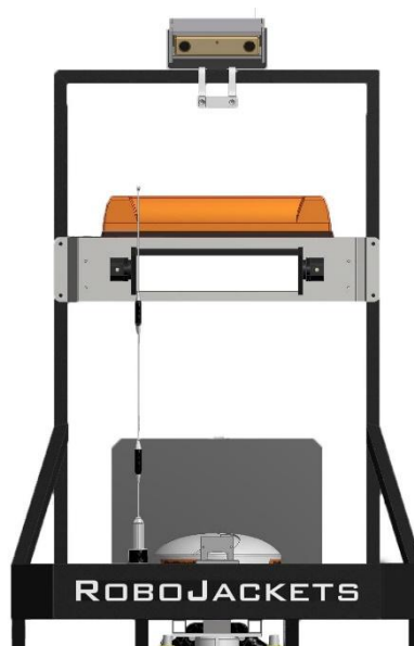
Figure 3. Mast and Related Equipment
