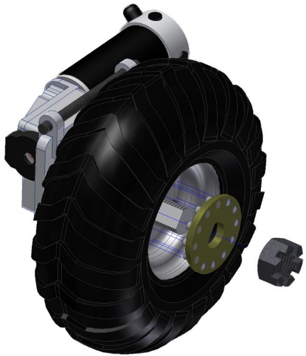
Figure 5b. Exploded View of Decoupling Mechanism Assembly
