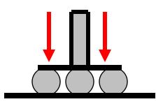
• Radial loads are applied from shaft to housing or support
