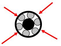
• Radial loads are applied from wheels to shaft
