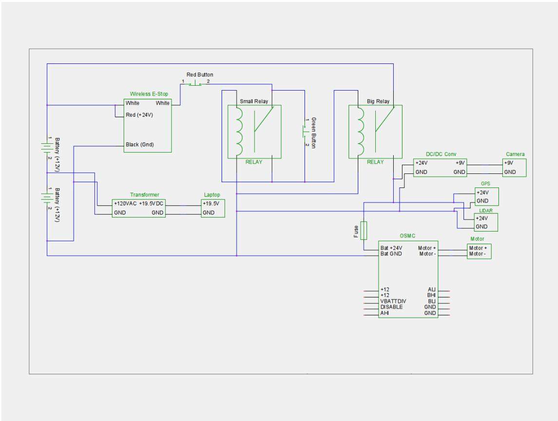
Figure 5: Power Schematic
