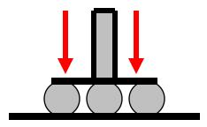
Radial loads are applied from shaft to housing or support
