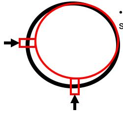
• Even though the shaft is off-centered, the set screw clamping force is effective
