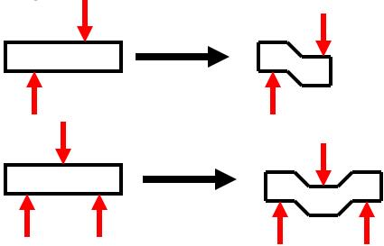
• Double shear setups reduce load on pins by 1/2
