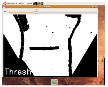
similar to grass are marked white and everything else is marked black. To account for various light conditions, the color for grass is found by averaging a small part of the image close to the robot which should contain grass. The grass color is also averaged over time to prevent fluctuations from things like dead grass. There is also a check to ensure that the grass color is somewhat similar to grass; if it is not, that frame is not included in the average.
