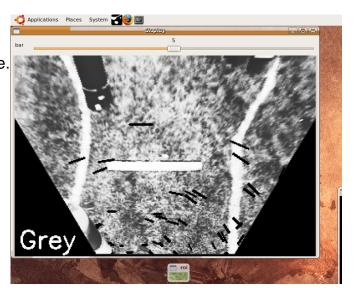
has been translated and rotated. We used the feature tracking software in OpenCV, another open source computer vision library. Using the matched features, we then find the most likely homography matrix, translation and rotation, between two images. The matched features often included several incorrectly matched points, so we used RANSAC, a nonlinear filter that is good at handling outliers, to choose the best homography matrix.
