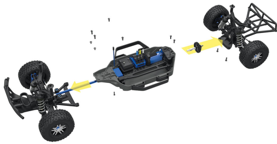
Fig. 1. Modularity of the Traxxas Slash 4x4 Design [1]
