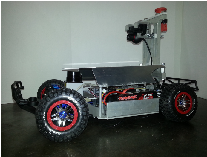
Fig. 3. Roll Cage Protecting Major Electrical Components
