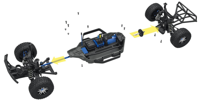
Fig. 1. Modularity of the Traxxas Slash 4x4 Design [1]
