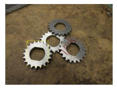
**Image Notes** 1. As your set screw starts approaching its shaft diameter, the system begins to function like a "D" bore shaft.
