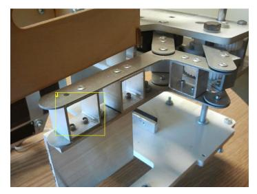
**Image Notes** 1. 1" square aluminum tubing is used on this robot as a spacing and structural element.
