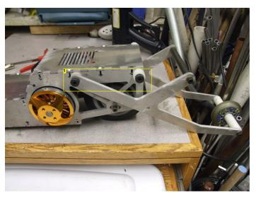
Image Notes 1. Straight RazEr's wheelie bar and its limit stop are both made with shoulder screws.
