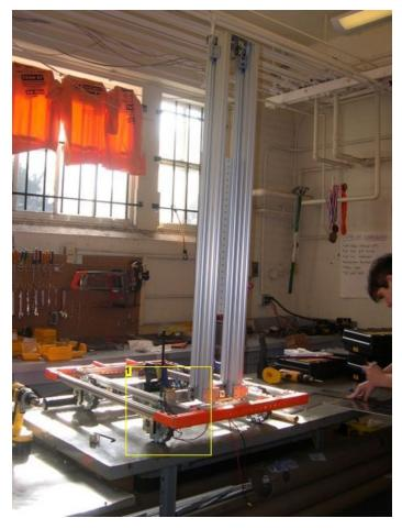
Image Notes 1. 80/20 and similar slotted extrusions are valued by robotics competitions for its ease of assembly.
