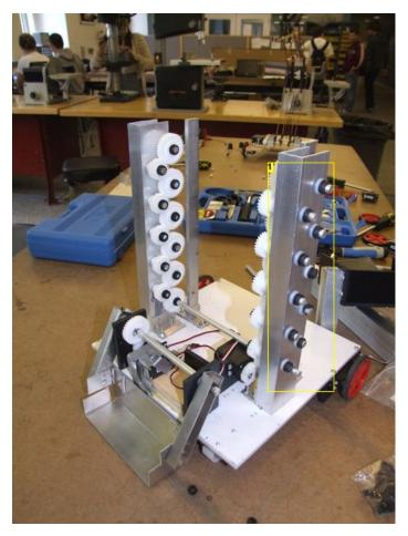
1. Live axles everywhere! These holes were drilled in one shot on a milling machine to guarantee the bushings lining up.
