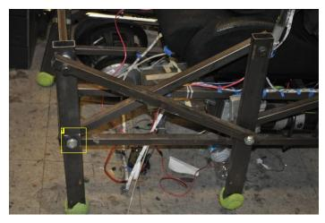
Image Notes 1. A locknut-based planar linkage.
