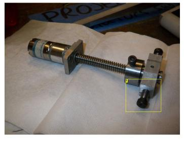
Image Notes 1. This weird little spring loaded trunion pulls on a mechanical linkage via shoulder screws.
