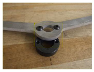
Image Notes 1. These "face mount" shaft collars basically hold Chibikart together.
