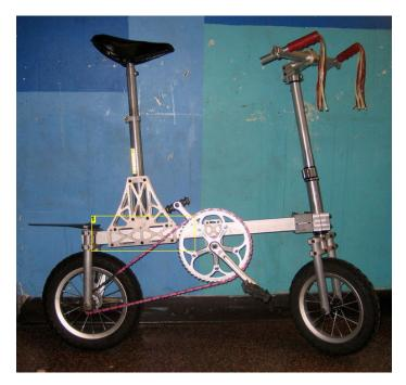
Image Notes 1. Don't know where things are going on your extrusion frame? Just clamp them in place with 2 plates.
