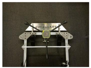
Image Notes 1. Chibikart's original steering handle was a machine vise handle, so I used a hex bore clamped-coupled into an aluminum tube for the steering shaft. It is
