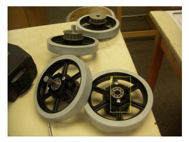
**Image Notes** 1. These pulleys were centered on the wheel axis with a 1/2" shaft, then 'starter dimples' drilled into the pulley using the premade wheel as a template.
