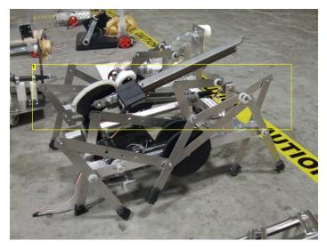
1. Unfortunately, this very well designed robot failed in execution because its legs were very poorly constrained, relying on not-so-tightened screws to maintain alignment. Proper use of fasteners is key to executing a robust design.
