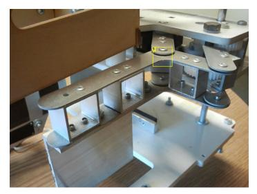
1. Notice the gap from the shim used. This robot is a good example of using symmetrical linkages - one set on top, and one set on bottom, to give double support.
