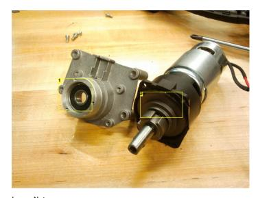
Image Notes1. This part is from a handheld circular saw, which is clearly a single-supported load. Is this the only bearing?2. Nope, the other one is integrated into the internal gearbox.
