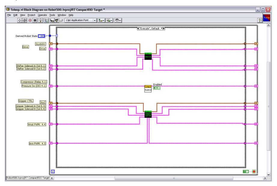
Robot\_Drive.VI - This module controls the Motors and shifters. The Joystick Axis control the motor with the Y-Axis being the speed and the X-Axis being the turn rate, the trigger button controls the shifter. If the button is pressed, we apply FALSE and TRUE to the solenoids, else, we apply TRUE and FALSE. That's all it takes to drive the robot with a dual speed gearbox.
