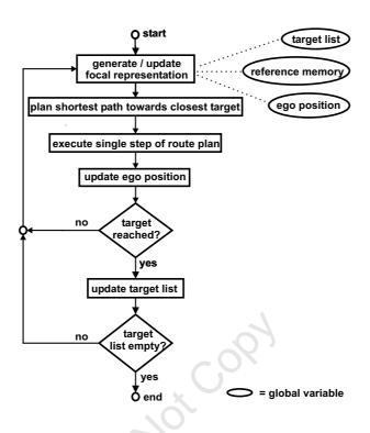
Figure 15. A generic flow chart of the fine-to-coarse planning heuristic.
