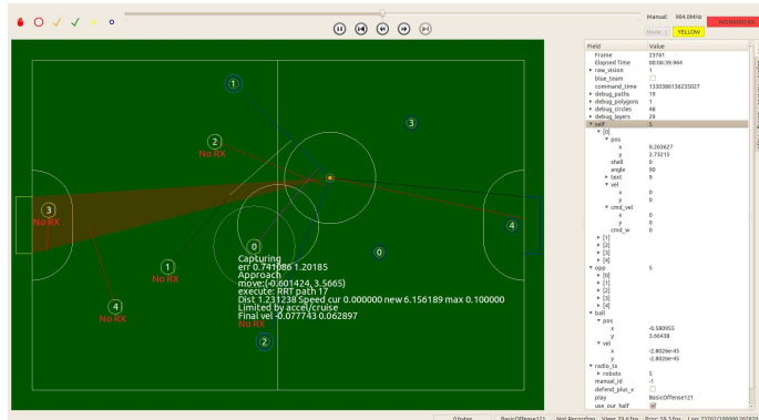
Fig 1: RoboJackets Soccer interface, showing play execution while under simulation.
