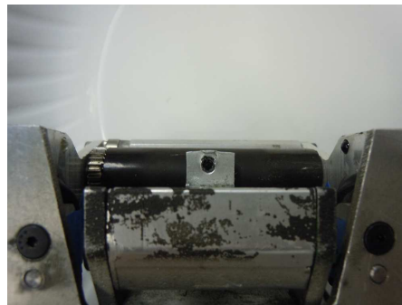
(b) Deformation in the kicker plunger
