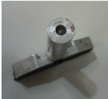
(a) Kicker plunger thread failure
